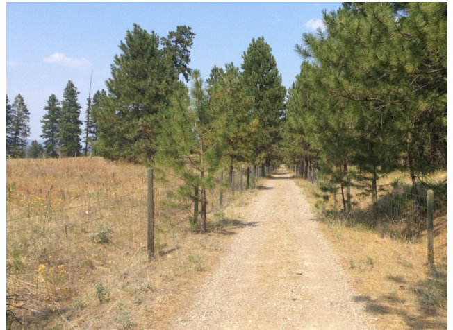
▼ Figure 40: Example of trail section near Rock Creek with vertical and horizontal clearance not suitable for large motorized vehicles and equestrian users, but suitable for most other non-motorized user groups
