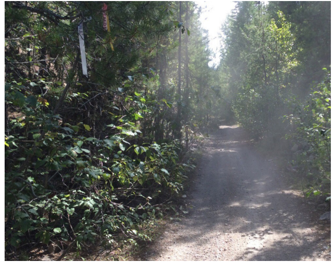
▼ Figure 40: Example of trail section near Rock Creek with vertical and horizontal clearance not suitable for large motorized vehicles and equestrian users, but suitable for most other non-motorized user groups
